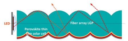
Figure 1 Light emitted by the LEDs is coupled into the fiber array guiding plate propagating in an interrupted chaotic whispering gallery mode.
