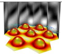
B) A plane wave is incident on a reflecting hexagonal grating. (Comsol©)
