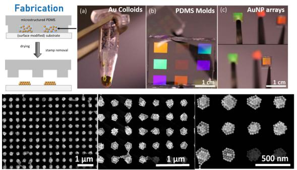
**Figure1**. Plasmonic crystals are readily fabricated within minutes without requiring complex lithographies. (a-c) Show the colloidal Au inks employed, the stamps used for the assembly and the resulting structures. The bottom images correspond to different magnification SEM of the crystals.
