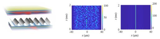
Schematic of a BAS-laser array with a PT-axisymmetric geometry with a bright and narrow output beam. Turbulent output in unmodulated EELs and localized field output in modulated EELs
