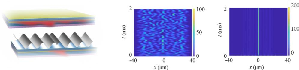
Schematic of a BAS-laser array with a PT-axisymmetric geometry with a bright and narrow output beam. Turbulent output in unmodulated EELs and localized field output in modulated EELs
